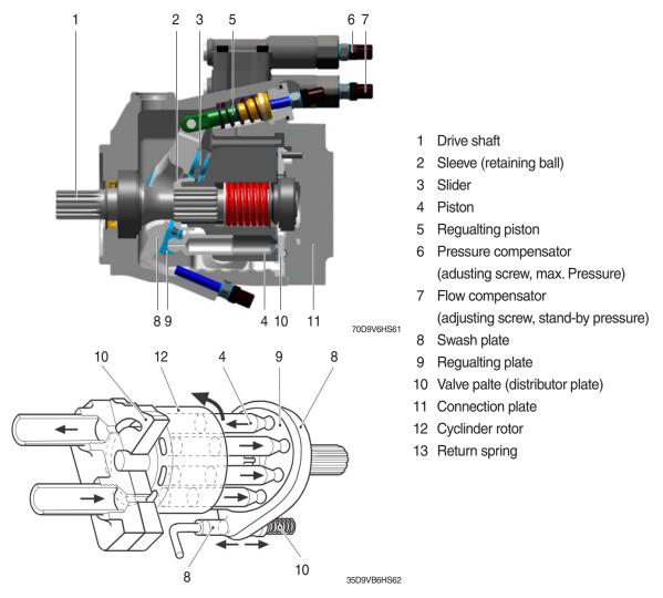
These pumps are the variable axial piston pump type and are controlled with load signals from the flow demand for each respective function. They pump oil with 9 pistons (4) that are located in a cylindrical cylinder block (cylinder rotor). The pistons (4) are tubular sleeves with a ball-shaped top. There are T-shaped sliders (3) on the piston top. The sliders are fixed in the swash plate (8).
