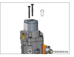
(8) Remove the gear pump section.
