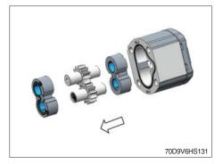
(10) Remove seal and anti-extrusion seal.
