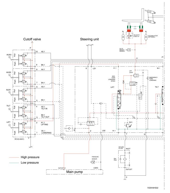
When the lift control lever is pulled back, the spool in the first block is moves to lift position. The oil from the main pump flows into main control valve through the priority valve. Then goes to the large chamber of lift cylinder by pushing the load check valve of the spool and lift lock valve.
