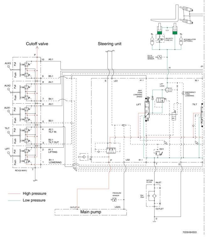
When the lift control is pushed forward, the spool in the first block is moved to lower position. The work port and the small chamber and the large chamber are connected to the return passage, so the forks will be lowered due to its own weight.
