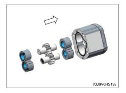
(17) Reassemble the gear pump section.
