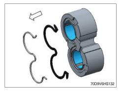
(11) Insert new seal and anti-extrusion seal.
