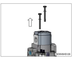
(8) Remove the gear pump section.
