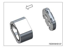
(16) Reassemble thrust plates and gears.
